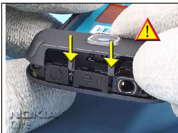
12. Fit the CAMERA COVER ASSY onto the B-COVER, paying attention to the correct position of the POWER KEY and the USB DOOR.
