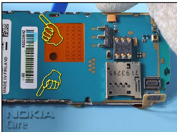
15. The PWB is secured with two hooks to the UI SHIELD ASSY. Gently unlock the PWB with the SS-93...
