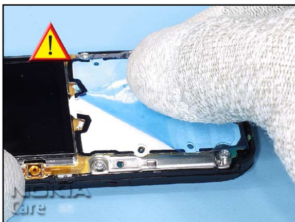
9. Carefully remove the protective film from the DOMESHEET.
