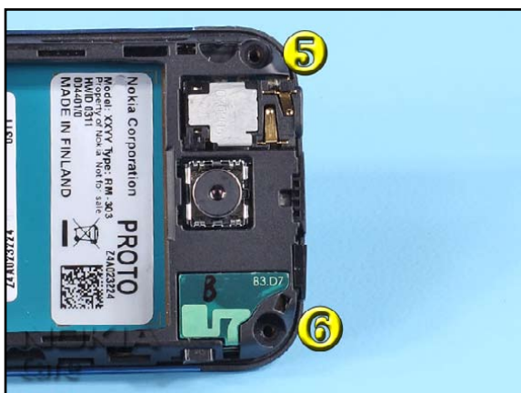
11. Insert new screws and tighten them with a torque of 21Ncm in the order shown.
