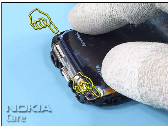
7. Secure the UI-SHIELD ASSY.
