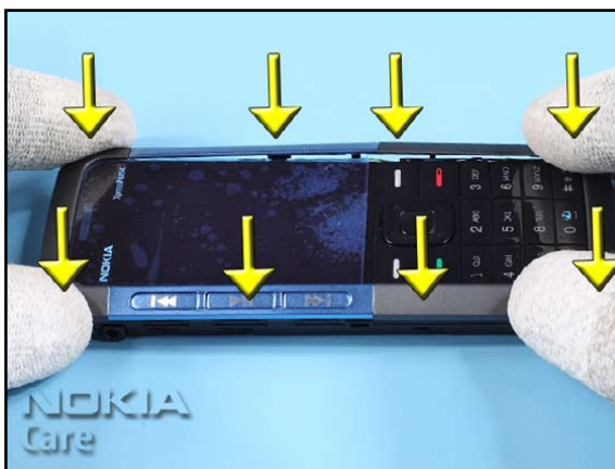
10. Align the A-COVER ASSY the B-COVER and gently close all snaps. Check that no gaps remain.
