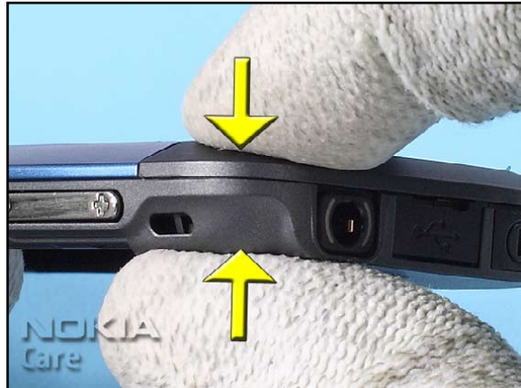
14. Secure also the other side of the CAMERA COVER.
