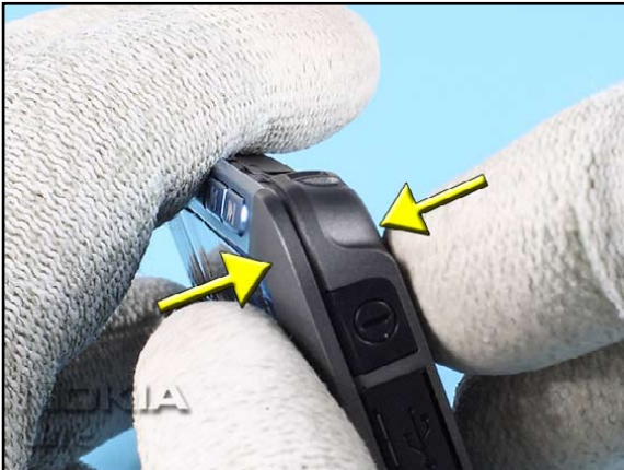
13. Press the CAMERA COVER ASSY and the B-COVER together.
